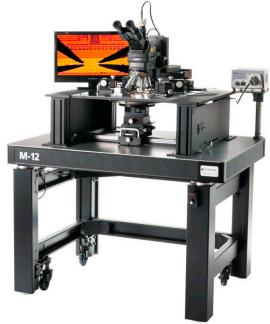
M-12 manual probe system configured above with a Rapid Advance wafer chuck, 300 mm chuck, fixed platen, DC manipulators, compound optics, CCTV system, test instrumentation mounted on a vibration isolation table - several configurations available.
