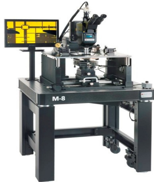
M-8 manual probe system with a Rapid Advance wafer stage, a 200 mm tilting chuck, a platen with linear lift, DC manipulators, compound optics, CCTV system mounted on a vibration isolation table - several configurations available.
